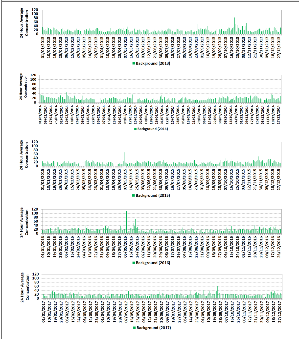
Figure 1: Five Years of Background Levels of the 24 Hour average Concentration of PM 10 (µg/m 3 )
